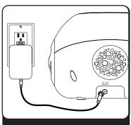
Attach AC adaptor cable to jack on back of the iH150 and plug the other end into a wall socket to play and charge iPod.
